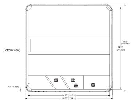
**NOTE:** Watkins Manufacturing Corporation recommends that the Tempo be installed on a minimum 4" (10.2cm) thick reinforced concrete pad or structurally sound deck able to support the "dead weight" found in the spa specification chart.
