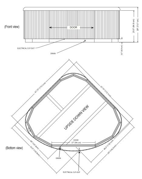
**NOTE:** Watkins Manufacturing Corporation recommends that the TX be installed on a minimum 4" (10.2cm) thick reinforced concrete pad or structurally sound deck able to support the "dead weight" found in the spa specification chart.
